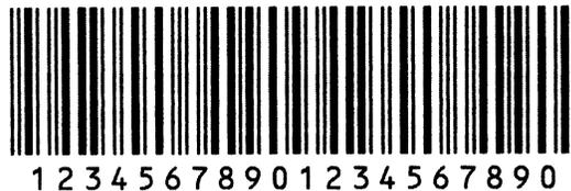
example 7: Interleaved 2 of 5, CD: Printer, HRI: none
